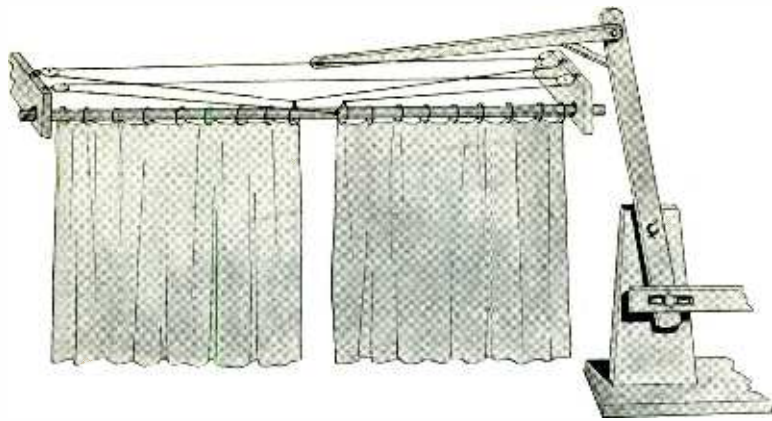
This is the standard two-curtain cord pull arrangement, except that both ends are fastened to the end of a swinging arm, which is actuated by a motor through a reduction gear
